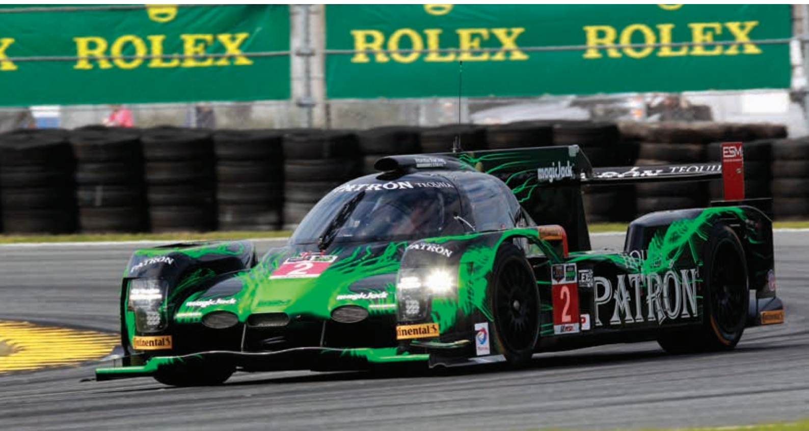
The distinctive twin holes in the car's nose channel air straight into the cockpit, saving weight and removing the need to fit an energy-draining air conditioning unit
