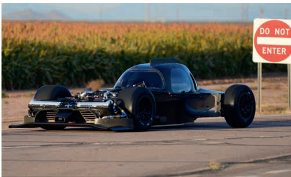
Above: The bottom half of carbon fibre tub has a distinct V shape to increase the volume of air passing through the car
