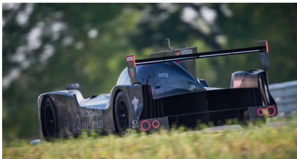
Nissan's GT-R LM NISMO racecar features a weight distribution of at least 65 per cent front, and 35 per cent rear
