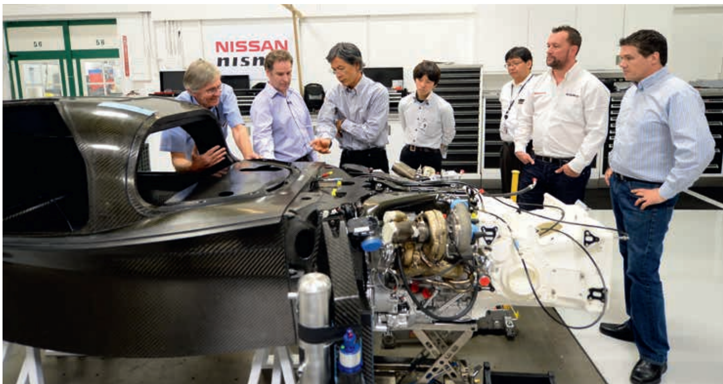
Above: The bottom half of carbon fibre tub has a distinct V shape to increase the volume of air passing through the car
